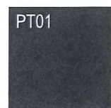
PAINT FINISH TO EXPOSED STEEL AND AWNING FASCIA- PFC (ALL EXTERNAL STEEL TO BE GALVANISED) COLOUR - COLORBOND - MONUMENT
